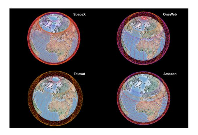
MIT researchers assess the data capacity of proposed satellite mega-networks from SpaceX (top left), OneWeb (top right), Telesat (bottom left), and Amazon (bottom right). Shown here are the satellite configurations of each network as specified in their filings. Credit: Massachusetts Institute of Technology
