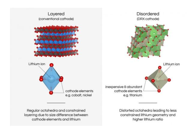
Illustration of a DRX cathode's "disordered" atomic structure (right) versus the "ordered" atomic structure of a conventional cathode. A disordered cathode structure can store more lithium - which means more energy - while allowing for a wider range of elements to serve as the transition metal. Credit: Berkeley Lab
