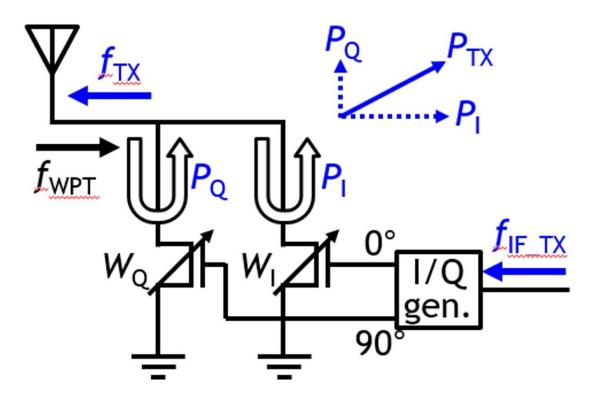
The vector-summing backscatter up-converts 4GHz I/Q signal and transmits at 28GHz. Credit: 2021 Symposia on VLSI Technology and Circuits
