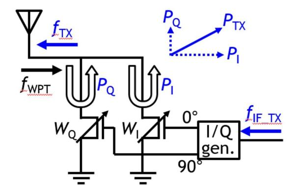
The vector-summing backscatter up-converts 4GHz I/Q signal and transmits at 28GHz. Credit: 2021 Symposia on VLSI Technology and Circuits
