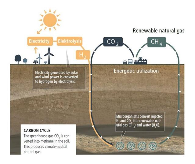
Carbon cycle: The greenhouse gas CO2 is converted into methane in the soil. This produces climate-neutral natural gas. Credit: RAG
