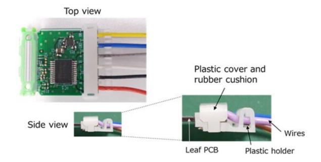
An example of wire connecter between motor control PCBs and motors. Credit: Toshiba Corporation
