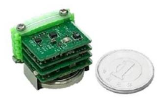
IoT module with the new connect technologies: The dimensions are typically 2 x 2 cm. The module consists of a sensor leaf PCB, microcontroller leaf PCB, Bluetooth leaf PCB, and a battery (CR2032) leaf PCB. Credit: Toshiba Corporation
