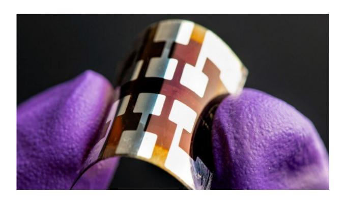
A solar cell made with perovskite, shown here, shows promise as an energy-efficient, scalable and longer-lasting way to create solar panels – and may be recycled for even greater sustainability. Credit: Dennis Schroeder/National Renewable Energy Laboratory
