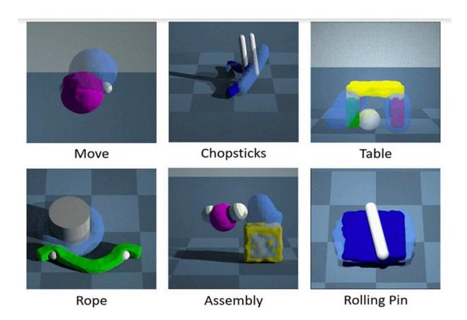
A new simulation environment, PlasticineLab, is designed to make robot learning more intuitive. Tasks like the ones pictured are designed to train agents to manipulate soft and deformable objects resembling those found in the real world. Credit: MIT-IBM Watson AI Lab.
