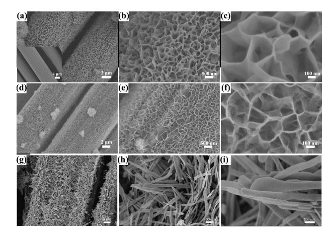
Figure 2. SEM images of (a-c) Co-Ni LDH/CC, (d-f) CoN-Ni<sub>3</sub>N/N-C/CC, and (g-i)VN/CC at different magnification. Credit: LI Kunzhen
