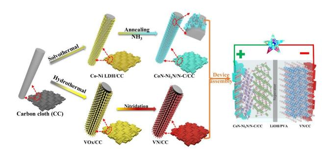
Figure 1. Schematic diagram of the formation process of CoN-Ni3N/N-C/CC, VN/CC, and the assembly of the flexible quasi-solid-state asymmetric supercapacitor device. Credit: LI Kunzhen
