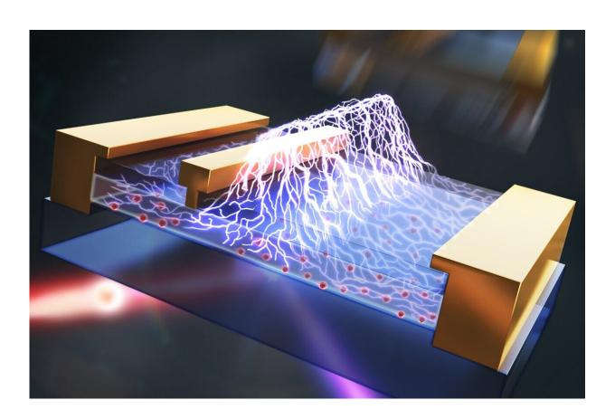
Quantifying electric fields in semiconductor devices: The schematic shows electric field distribution in the channel of a GaN transistor; laser beams highlight the second harmonic generation (SHG) nature of the technique. Credit: Yuke Cao
