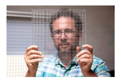
Dr Gianluca Memoli demonstrating one of Metasonixx's transparent panels which are designed to allow air through. Credit: University of Sussex
