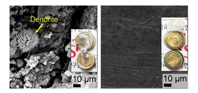
Top-view SEM images and photographs (inset) of plain-Li, and Li@p-PCL electrodes after cycling tests with LilLi symmetrical cells at 1.0 mA cm-2 and 1.0 mAh cm-2. Credit: Korea Institute of Science and Technology (KIST)
