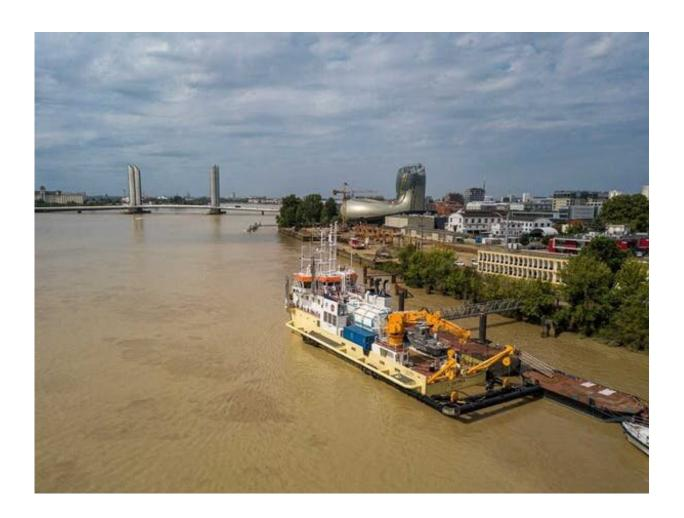
In 2020, Bordeaux's port was fitted out with an LNG-powered dredger, which requires less energy and is more environmentally friendly, thanks to its water injection-dredging mechanism. Credit: Delphine Trentacosta, Author provided
