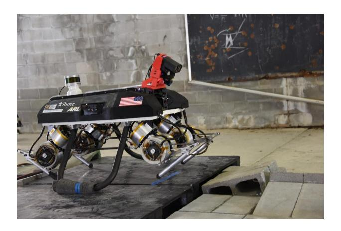
The Legged Locomotion and Movement Adaptation, or LLAMA, is an autonomous quadruped mobility research platform system patterned after a working dog and similar animals. Army researchers designed it to work alongside soldiers, lighten physical workloads, and increase mobility, protection and lethality. (U.S. Army). Credit: U.S. Army Photo
