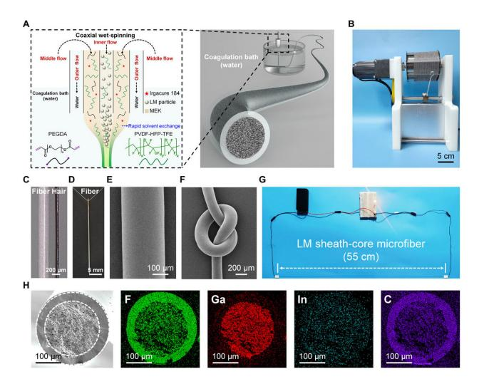
Preparation of LM sheath-core microfibers. (A) Schematic setup and the main components for the coaxial wet-spinning process for producing LM sheath-core microfibers. (B) A single as-spun fiber with the length of 380 m was collected on a continuously winding collector. (C) Microscopic images of LM sheath-core microfiber and human hair. (D) Photo of the microfiber threaded into a needle. (E) SEM image of the external surface of the microfiber. (F) SEM image of a
