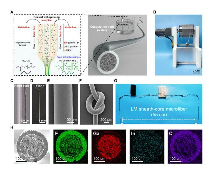
Preparation of LM sheath-core microfibers. (A) Schematic setup and the main components for the coaxial wet-spinning process for producing LM sheath-core microfibers. (B) A single as-spun fiber with the length of 380 m was collected on a continuously winding collector. (C) Microscopic images of LM sheath-core microfiber and human hair. (D) Photo of the microfiber threaded into a needle. (E) SEM image of the external surface of the microfiber. (F) SEM image of a
