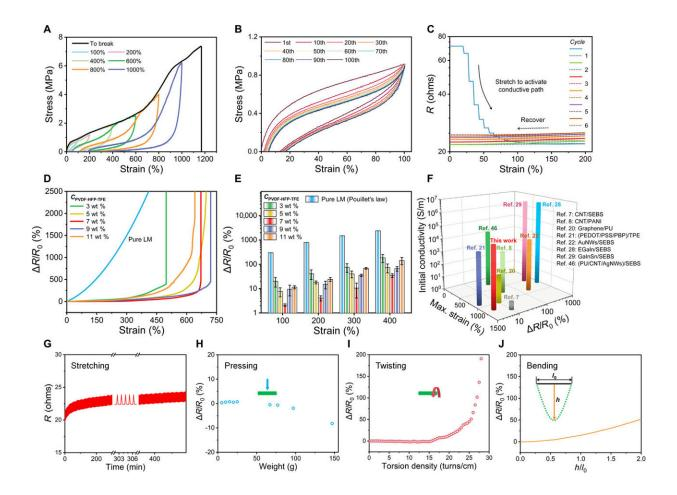
Mechanical properties and strain-insensitive conductance of LM sheath-core microfibers. (A) Tensile stress-strain curves of LM sheath-core microfibers and the hysteresis loops measured at increasing strains (stretching rate: 20 mm/min).
