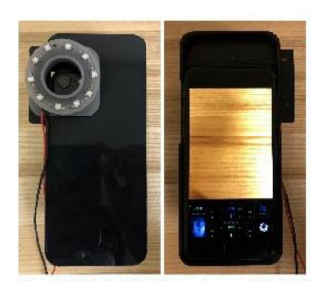
Photographs of the modified smartphone that the researchers used to capture LED-illuminated RGB images of skin and oral cavities. Credit: He et al., Optics
