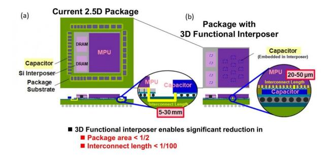
The new interposer design with an embedded capacitor provides a notable reduction in area requirements and interconnect length, leading to lower wiring resistance and parasitic capacitance. MPU: Microprocessing unit; DRAM: Direct random-access memory. Credit: The 2021 IEEE Electronic Components and Technology Conference
