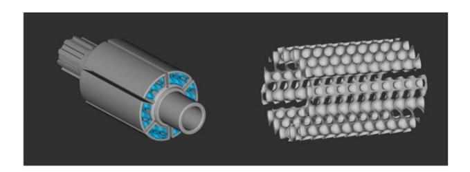
By using computer-aided design and additive manufacturing, developers can improve the performance characteristics of geothermal tools, such as this optimized rotor design, and reduce production cost. Credit: ORNL, U.S. Dept. of Energy
