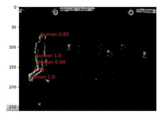
Imec's end-to-end spiking approach at work. Local feature detection forms the first layer for a more complex semantic build-up. Credit: IMEC
