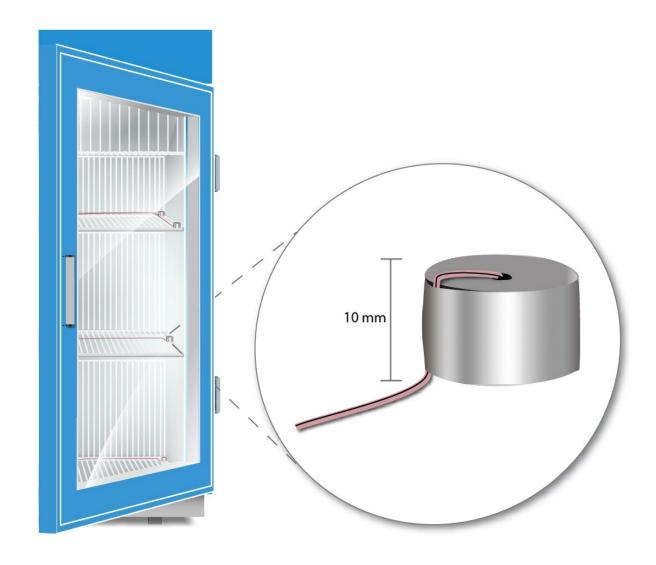
The VSD (vaccine simulation device) illustrated here was designed by the standard committee as a stand-in for a real vaccine vial. Each device is small — only 10 mm tall — and made of aluminum. The devices will be used by laboratories to evaluate the performance of medical fridges and freezers being considered for NSF certification. Credit: Kristen Dill/NIST
