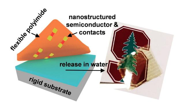
Illustration of transfer process for 2D semiconductor with nanopatterned contacts (left) and photograph of flexible transparent substrate with transferred structures (right). Credit: Victoria Chen/Alwin Daus/Pop Lab
