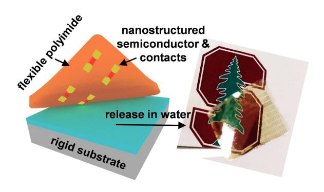
Illustration of transfer process for 2D semiconductor with nanopatterned contacts (left) and photograph of flexible transparent substrate with transferred structures (right). Credit: Victoria Chen/Alwin Daus/Pop Lab
