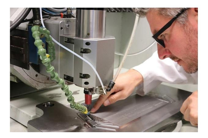
Udo Eckert, Group Leader Microsystems Manufacturing & Technical from the Functional Surfaces and Micromanufacturing department at Fraunhofer IWU, tests the finishing of a milled tool to be used in bipolar plate production for fuel cells at the micromachining center of Fraunhofer IWU. Credit: Fraunhofer IWU
