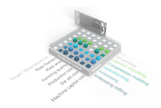
Visualization of the technology toolkit: The higher the column, the better that forming process scores on a particular parameter. Credit: Fraunhofer IWU
