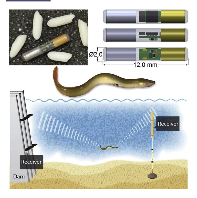
The acoustic tag sends a signal every five seconds, which is picked up by receivers that can be as far away as a football field is long. These receivers can be placed on dams to track passage or stand alone to track migration. (Illustration: Pacific Northwest National Laboratory)
