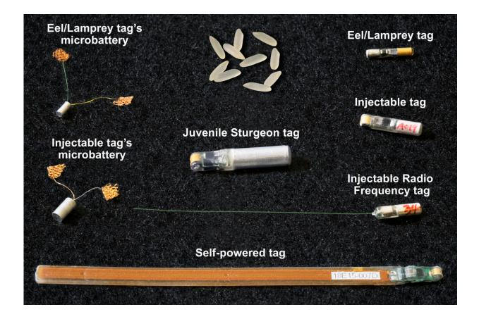
The eel/lamprey battery (top left) and tag (top right) relative to existing, commercially available technology. (Photo: Pacific Northwest National Laboratory)
