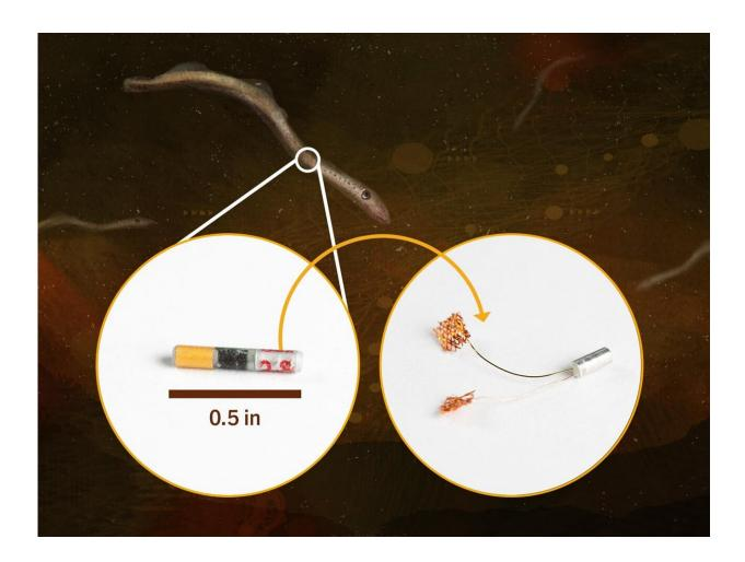
The new, super small acoustic tag (left) powered by a microbattery the size of a grain of rice (right), with twice the power of a household AAA battery. This tag provides new insight to sensitive species, such as Pacific lamprey. Credit: Stephanie King | Pacific Northwest National Laboratory
