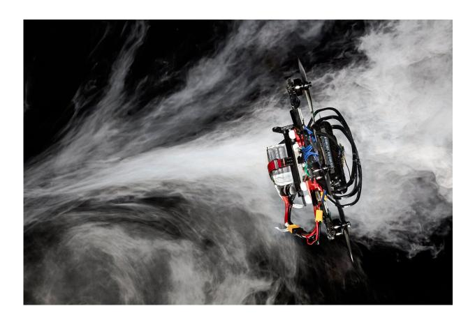
A drone flying through smoke to visualize the complex aerodynamic effects. Credit: Robotics and Perception Group, University of Zurich
