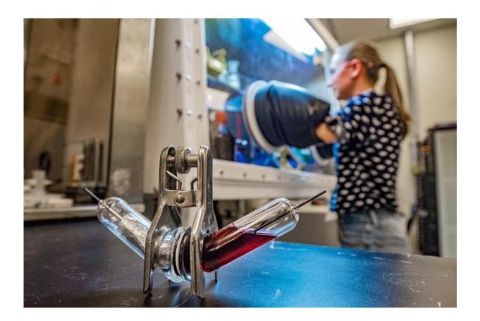
Postdoctoral researcher Martha Gross works in an argon glove box with a test battery cell illustrating a lab-scale sodium iodide battery. The Sandia National Laboratories research team developed a new sodium iodide catholyte solution (purple liquid) and a special ceramic separator to allow the molten sodium battery to operate at 230 degrees Fahrenheit (110 degrees Celsius). Credit: Randy Montoya/Sandia National Laboratories
