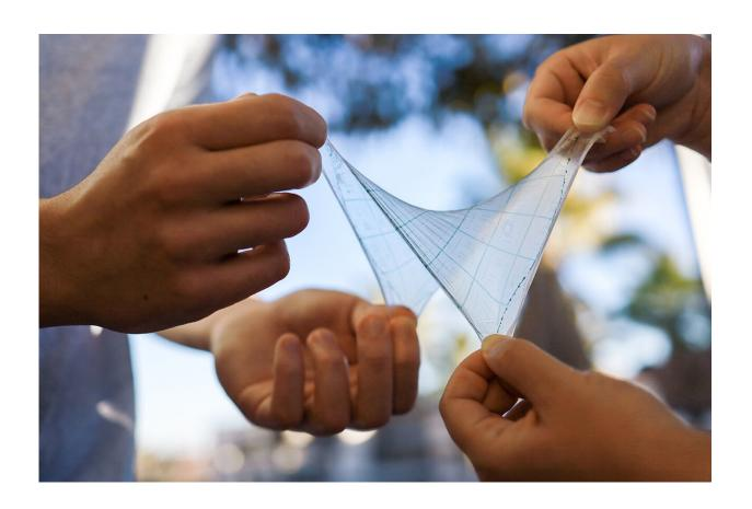
Lab mates in the Bao Research Group at Stanford demonstrate the flexibility and stretchability of their artificial skin made using their newly created printing method. Credit: Yuqing Zheng
