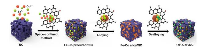
Schematic representation of the preparation of the microstructured FeP-CoP embedded nitrogen doped carbon electrocatalyst that is at the heart of the new electrolyser. Credit: HIMS
