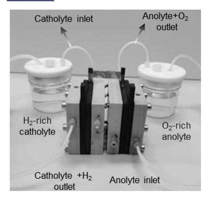
Bench scale prototype of the membrane-free water electrolyser. Credit: HIMS
