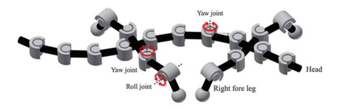
The simulated salamander model. The trunk has 10 rotary joints and each leg has two rotary joints. Credit: Ishiguro-Kano lab
