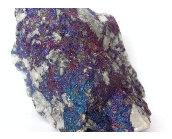
A sample of copper hosted in a quartz vein in the form of a mineral called chalcopyrite. When exposed to air, the surface oxidises to create this metallic 'peacock' lustre. Credit: Marek Novotňák / Wikimedia Commons
