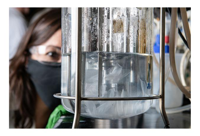
An NREL researcher observes visible changes in bioreactors used to test enzymatic degradation of PET plastic. In reactors loaded with less enzyme, the liquid appears unclouded and the plastic remains transparent. In reactors loaded with more enzyme, the liquid is cloudy and the plastic becomes opaque, as shown here. Credit: Dennis Schroeder, NREL
