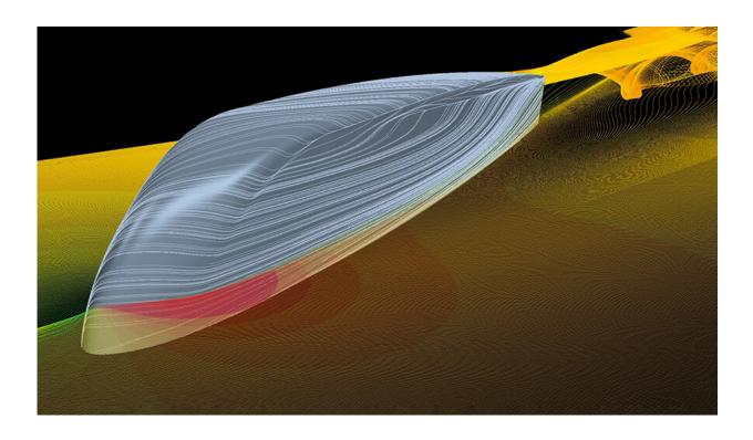
The velocity streamlines of the model, developed using computational fluid dynamics simulations on LLNL's supercomputers. Credit: Lawrence Livermore National Laboratory
