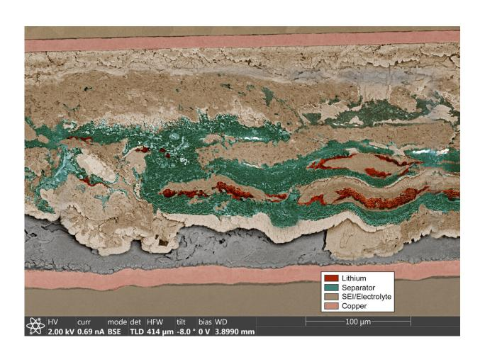
In this new, false-color image of a lithium-metal test battery produced by Sandia National Laboratories, high-rate charging and recharging red lithium metal greatly distorts the green separator, creating tan reaction byproducts, to the surprise of scientists. Credit: Katie Jungjohann
