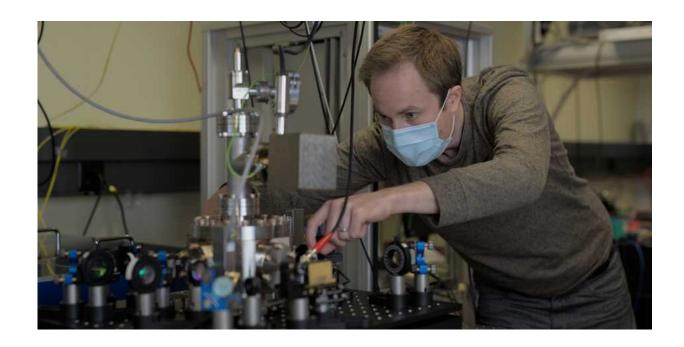
Dominik Husmann adjusts the optical setup used to generate a precise reference frequency based on an infrared laser. Credit: METAS
