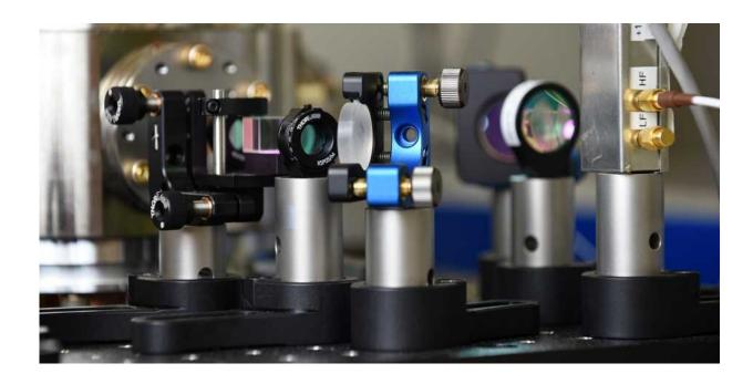
Close-up of the optical components used to stabilise the light of the infrared laser for the precise reference frequency. Credit: METAS
