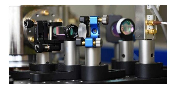
Close-up of the optical components used to stabilise the light of the infrared laser for the precise reference frequency. Credit: METAS
