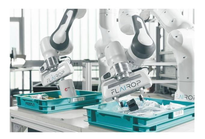
In the FLAIROP research project, autonomous robots process articles at several picking stations by means of gripping and transferring. Credit: Amadeus Bramsiepe, KIT
