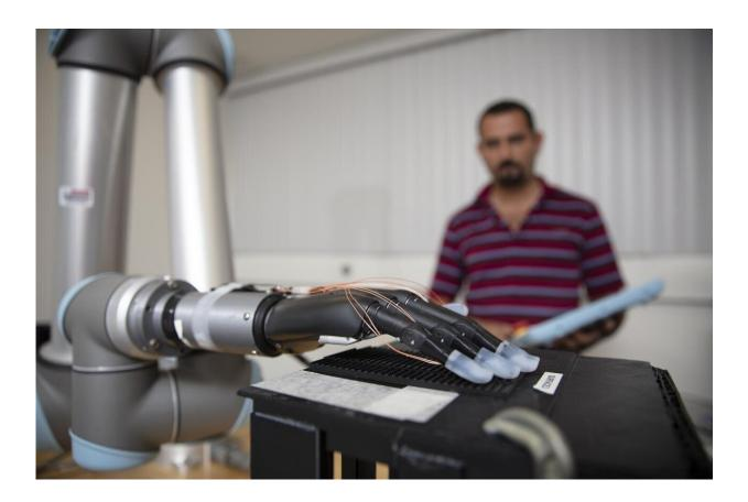
Researchers used individual fingertips fitted with stretchable tactile sensors with liquid metal on a prosthesis attached to a robotic arm. Credit: Alex Dolce, Florida Atlantic University
