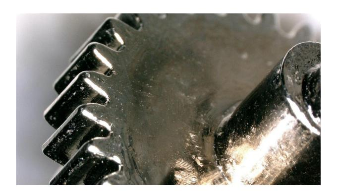
Most metallic glass alloys form a hard, smooth surface. This gives metallic glass gears a long lifetime without the need for liquid lubricants, making them appealing for NASA robotics that operate in cold environments, where lubricants need to be warmed before operations. Credit: NASA
