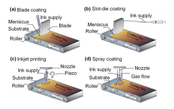
Scalable methods for PSCs deposition: (a) blade-coating, (b) slot-die-coating, (c) inkjet printing, and (d) spray-coating. Credit: Science China Press
