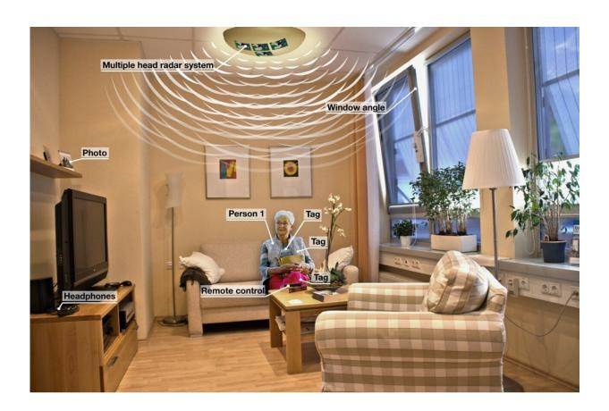
The passive tags can be unobtrusively integrated into everyday objects such as items of clothing. Radar modules on the ceiling detect the position and the movement of the tags. Credit: Fraunhofer-Gesellschaft
