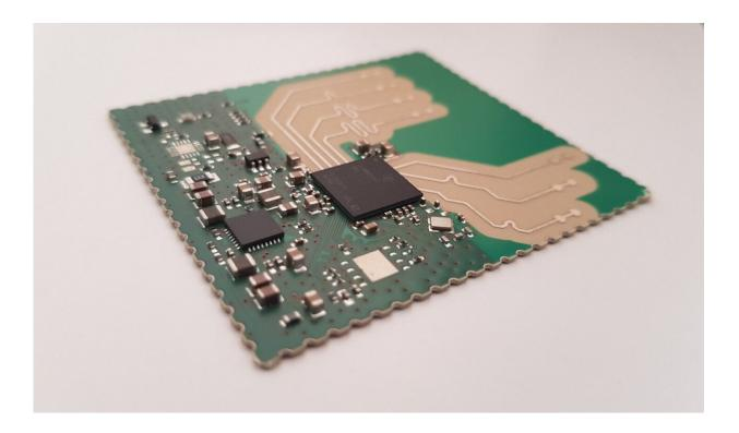
Up to nine send/receive modules like these are integrated into the lamp structure. In this arrangement, they cover the entire room. Credit: Fraunhofer-Gesellschaft
