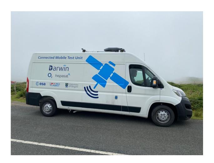
A vehicle that remains continuously connected even when in remote areas is being road tested in Cornwall in the south west of the UK. The test vehicle will use ubiquitous communications technology to switch seamlessly between 5G and satellite networks as required. The technology was developed by Darwin Innovation Group, in collaboration with mobile telephone operator Virgin Media O2, satellite operator Hispasat, cloud data company Amazon Web Services, the
