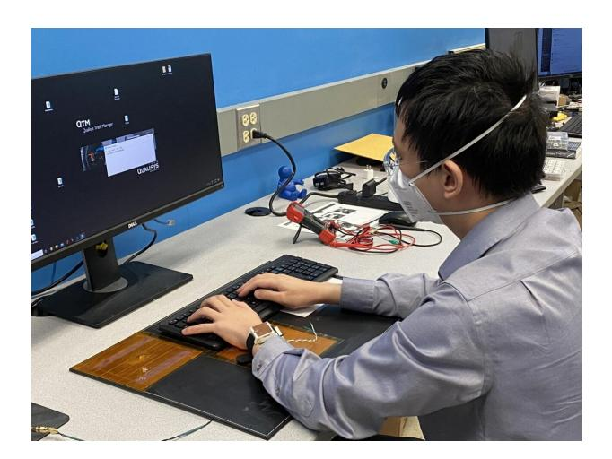
Sunghoon Ivan Lee demonstrates how the wearable device is charged through his left forearm's contact with the power transmitter below the keyboard. Credit: UMass Amherst
