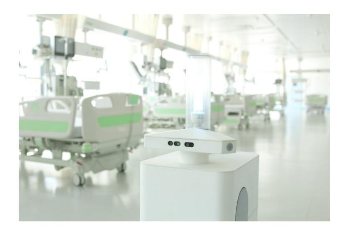
Smart functional robot that realizes simultaneous disinfection of both air and object surface developed by HFIPS researchers. Credit: ZHANG Wen
