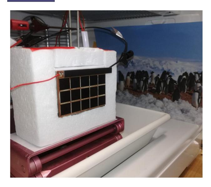
Efficiency increases, when the photovoltaic module is in close contact with the wall of the electrolysis tank. Credit: M. Kölbach/HZB
