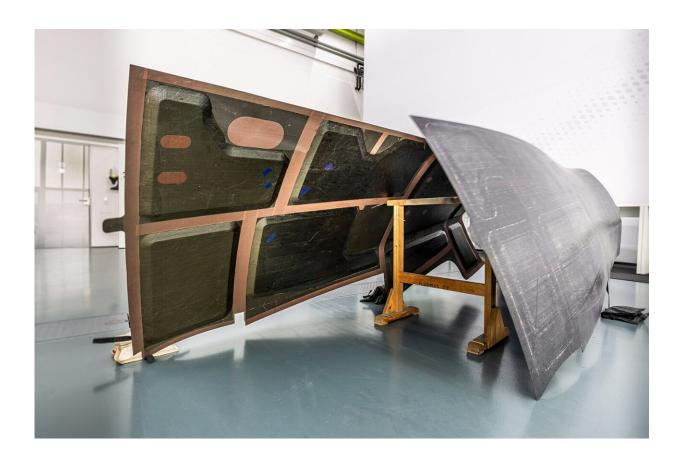
The cured side shells, ready for installation in the RACER helicopter prototype. The cured side shells, ready for installation in the RACER helicopter prototype. Credit: Fraunhofer-Gesellschaft
