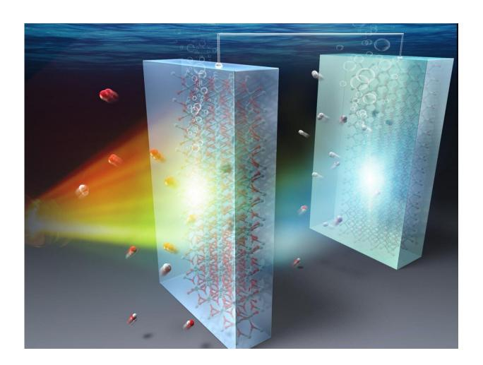
The use of a semitransparent TiO<sub>2</sub> photoanode allows the SiC photocathode to make use of the transmitted light. Using photocatalysts with different energy gaps results in increased conversion efficiency. Credit: Image courtesy: Masashi Kato from Nagoya Institute of Technology.
