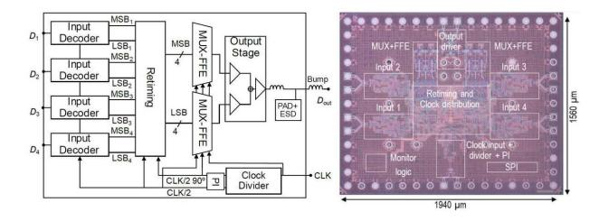
(Left) Block diagram and (right) die micrography of the 4:1 PAM-4 serializer chip with mixed-signal FFE, as presented at 2021 CICC. Credit: IMEC
