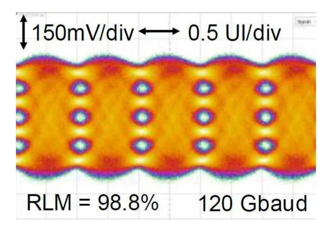
PAM-4 eye diagram at 120Gbaud on a flip-chipped sample with the FFE
