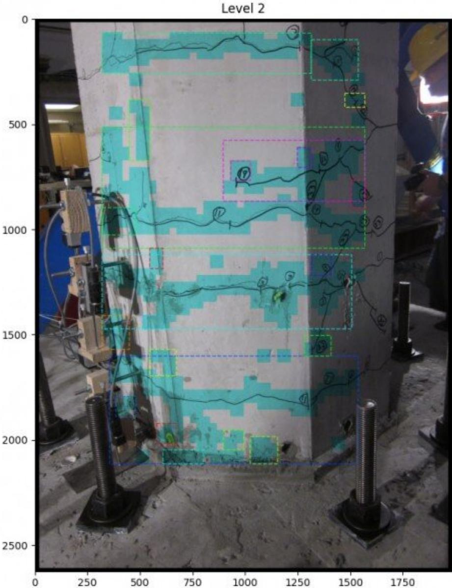
This image shows how the vision software automatically detects cracking in a reinforced concrete bridge column. Credit: South Dakota State University
