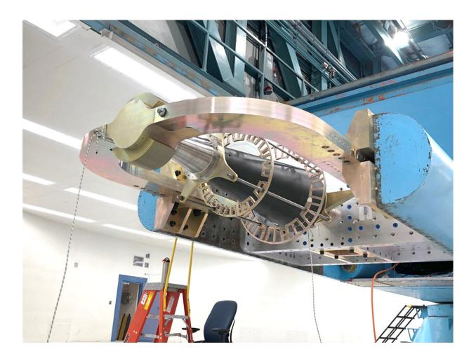
An experimental test system is mounted on the centrifuge arm prior to combined environments testing at the Sandia National Laboratories Superfuge/Centrifuge Complex in Albuquerque, New Mexico. Credit: Byron Demosthenous
