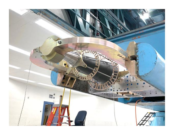
An experimental test system is mounted on the centrifuge arm prior to combined environments testing at the Sandia National Laboratories Superfuge/Centrifuge Complex in Albuquerque, New Mexico. Credit: Byron Demosthenous
