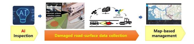
Overall flow of the developed automatic pothole detection system. Credit: Korea Institute of Civil Engineering and Building Technology (KICT)
