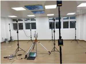
Real-time measurement of PM concentration inside the classroom in the testbed. Credit: Korea Institute of Civil Engineering and Building Technology (KICT)
