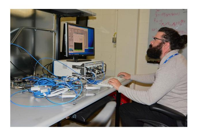
Mathematician Jacob Rezac uses a NIST modeling technique to find configurations that enable Wi-Fi and Bluetooth devices (located amid the blue wires) to share communications channels. Credit: Coder/NIST
