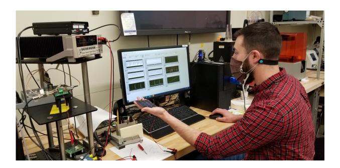
NIST researcher Andrew Shore holds a miniature high efficiency solar device as it charges a sensor using indoor light as an energy source. Credit: NIST
