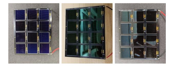
NIST researchers tested miniature solar modules made of three different materials under artificial light. The modules (from left to right) were made of silicon, gallium arsenide and gallium indium phosphide. Credit: NIST
